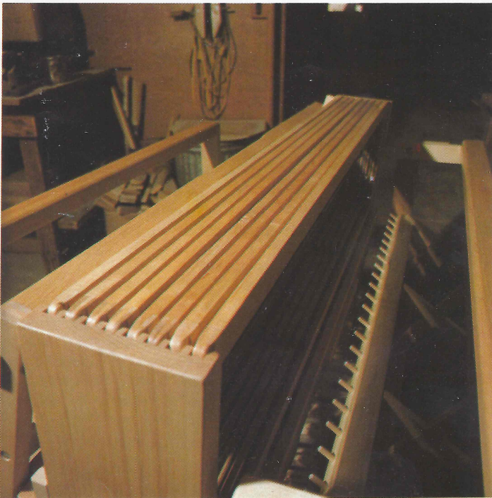
Harness frames which lift the pattern threads.
