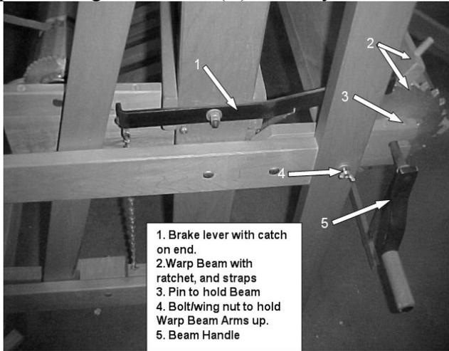
1. Brake lever with catch on end.
