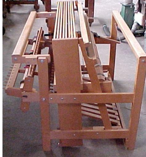
Older Compact Loom with "open" Warp Beam.
