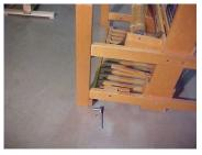
Step 3: Put the warp beam on. Secure with the rivet pins.
