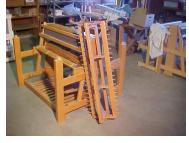
Step 4: Put the front top beam (breast beam) and the top back beam on. They are often marked inside the square mortise hole. (For example RF for right front.) The beams are usually interchangeable too.
