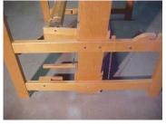
Step 2: Put the treadles on. There are pins on the back side of the lower front legs to align the treadle bar. Make sure the <u>back of the treadles</u> are on top of the treadle rest. Because of the brake treadle the treadles can only go on one way. Secure them with the 1/4" nut and washer. Once you have the treadles on, hook up the chain in the back for the brake release.
