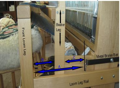
Using the above measurements make a part about 3/4" thick and a couple of inches wide and length A long. The photos label this part A.
