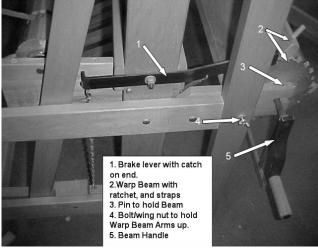
Older Compact Loom Brake system and "closed" (solid) Warp Beam.
