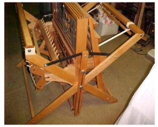
**COMPACT series loom:** These looms were designed to have the Warp Beam taken off and the arms that hold it swing down. The cross beam above it (Top Back Bar) is on arms that swing up. Doing these things allows the loom to
