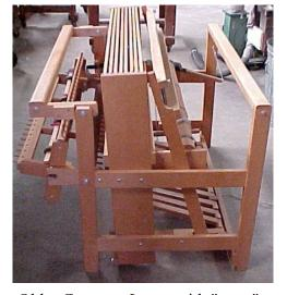
Older Compact Loom with "open" Warp Beam.
