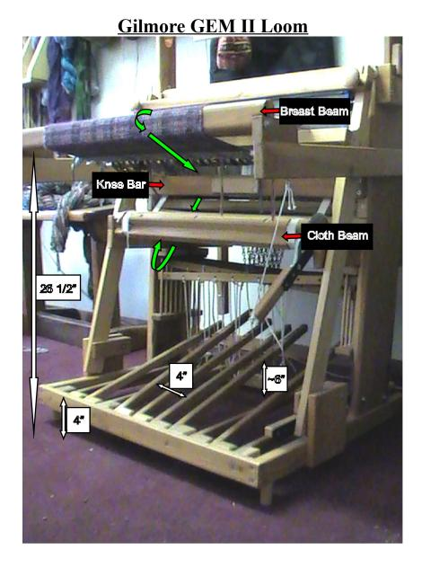
The GEM II is a studio loom made to be very sturdy and portable. It is designed so a weaver can weave at it with a chair. Woven material comes across the weaving area, around the Breast Beam, around the Knee Bar, and down to be wrapped on the Cloth Beam (Green line in photo). This keeps the woven material well above even tall weaver's legs.
